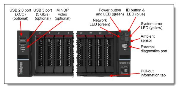
Figure 33. Front operator controls are on the left and right side of the server
