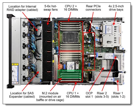
Figure 6. Internal view of the ThinkSystem SR650 V4
