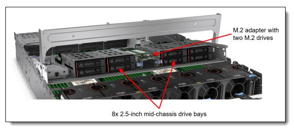
Figure 16. Mid-chassis drive bays
