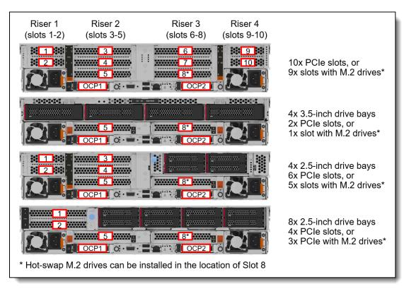
Figure 25. PCIe slots with rear drive bays
