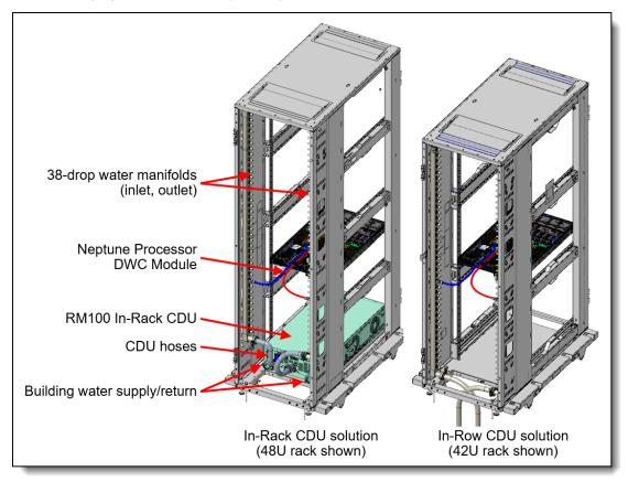
Figure 38. Water manifold connections
