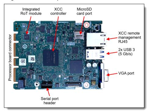
Figure 32. System I/O Board
