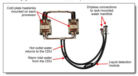
Figure 9. Lenovo Processor Neptune Core Module
