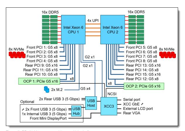
Figure 7. SR650 V4 system architectural block diagram
